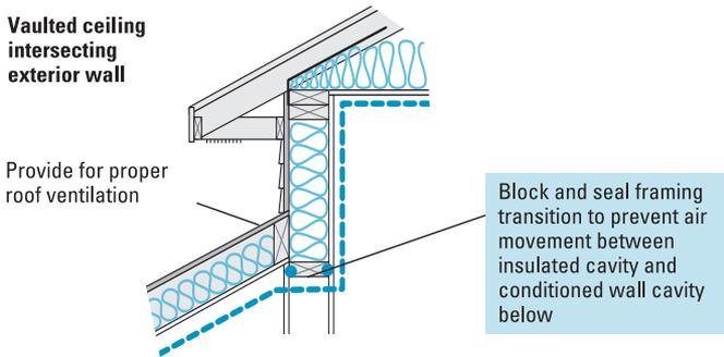
The lack of draftstop blocking in typical split-level details is another large leak. Be especially careful around stairways framed near these areas in “Tri-level” homes.
