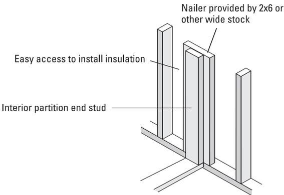
Vertical nailing stock can also be replaced by drywall clips to support drywall.
