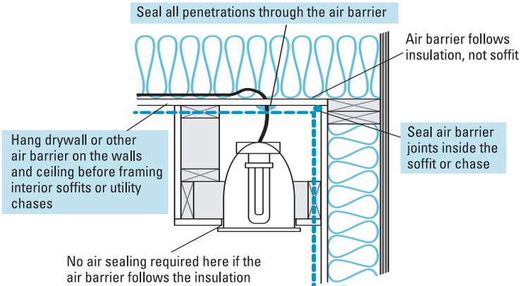
Dropped soffits are commonly built with direct air paths from inside interior walls into attics. When recessed lights are installed, heat from the lights drives air leakage even faster. Installing air barriers before framing the soffit requires coordination of framing crews and materials.
