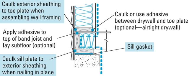
Remember to caulk or tape vertical seams between sheathing panels.
