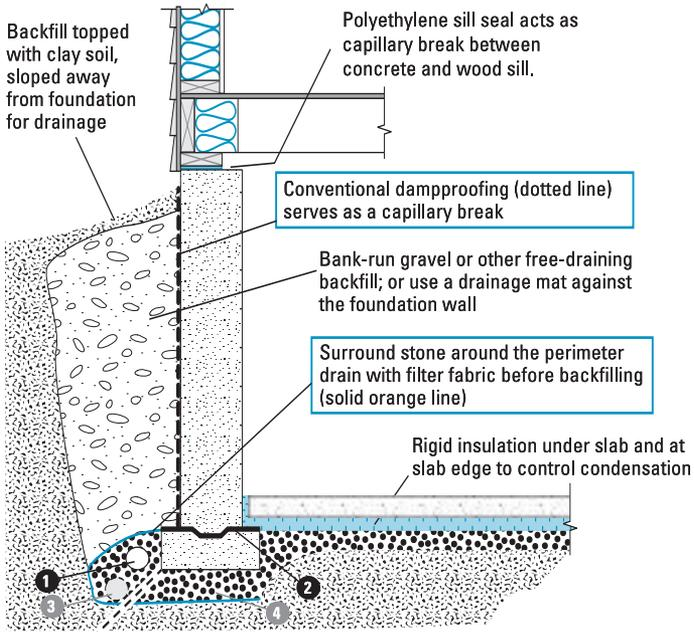
**1** Perforated drain pipe at footing level, drains downhill to daylight or to sump pit inside basement
